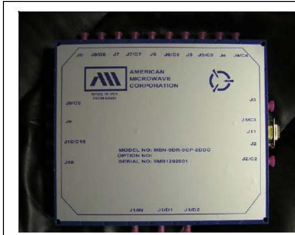
Operating at L-Band, this SP9T solid state switch offers 1.6dB Insertion Loss, >45dB Isolation, better than 1.5:1 VSWR, TTL control and handles up to 100 Watts CW. This part features a dual directional coupler on the input and each of the 9 outputs has a coupled port (26dB).
