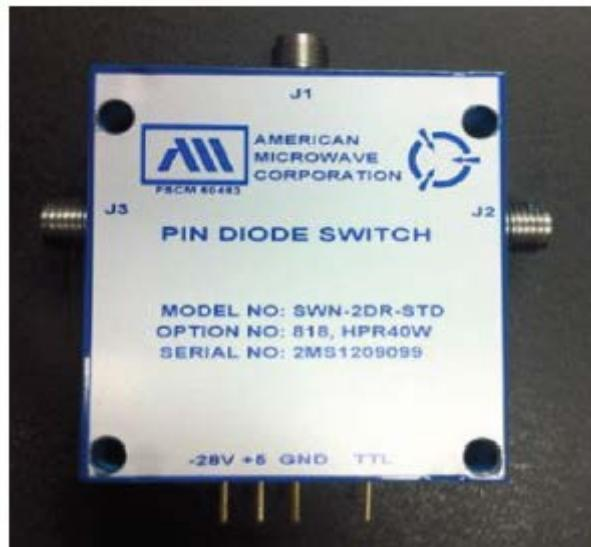
Model SWN-2DR- STD is a SPDT solid state reflective switch capable of operating from 8-18 GHz and can handle 40W of CW power. The switch has a maximum Insertion Loss of 2 dB, VSWR of 2.0:1 maximum and an isolation of >40 dB. It has a maximum switching speed of 150 nSec. Switching rate is 500 KHz max. Input and output connectors are SMA (F) and solder pins for TTL and power supplies. Size is 1.6"(L) X 1.72(W) X 0.62"(H).
